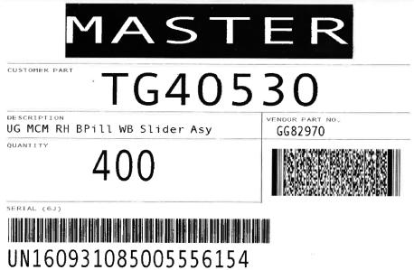
All products received by ABC must contain a serial number that is clearly identified on each label and every container. Suppliers can add date codes etc. within their allotted space.
